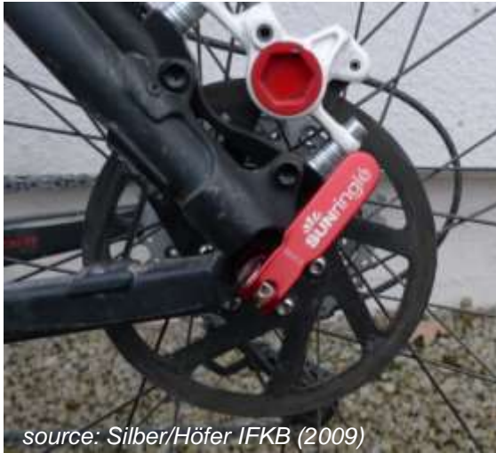
Brake rotor for bicycles after 150 km test run
