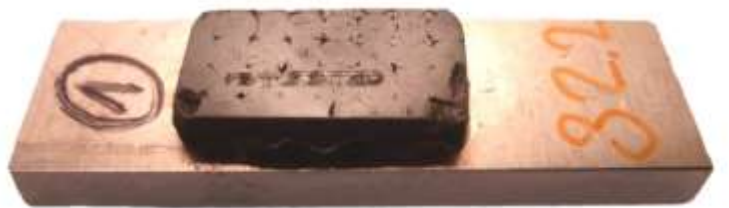
Volumetric wear track on B_f/SiOC 1000 °C specimen
