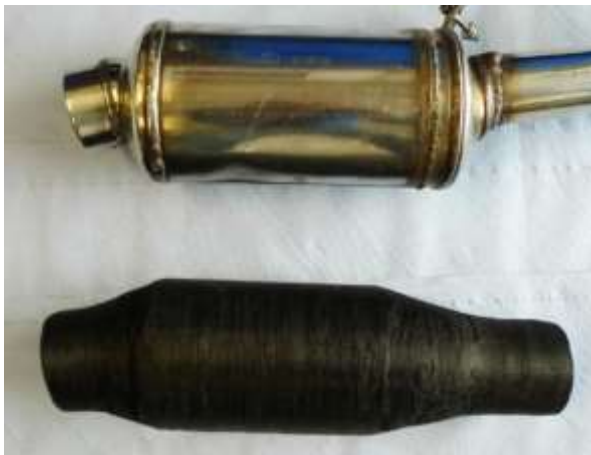
Exhaust silencer demonstrator: weight saving >65 % vs. stainless steel
