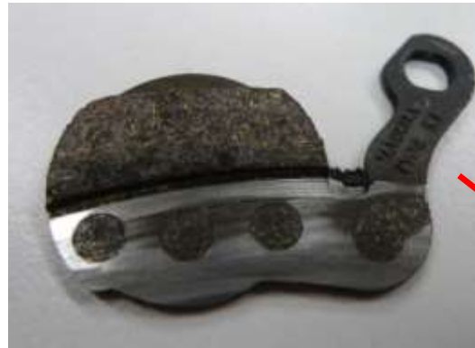
organic brake pad after 150 km test run with B_f /SiOC rotor
